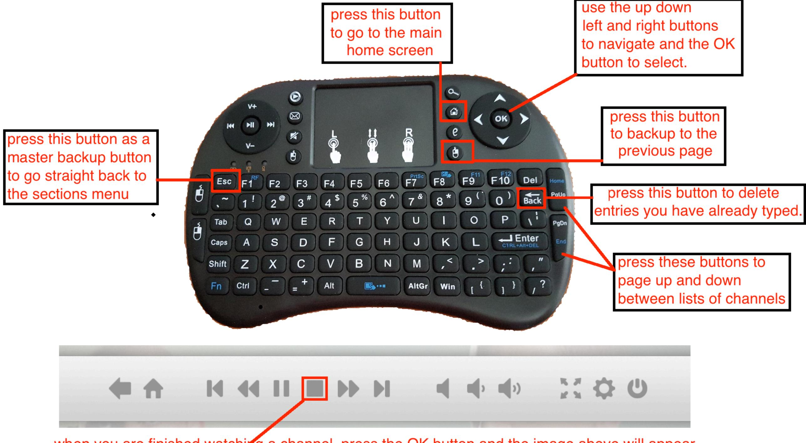
when you are finished watching a channel, press the OK button and the image above will appear. Then click on the SQUARE button to stop the stream or click on the PAUSE button to pause.
